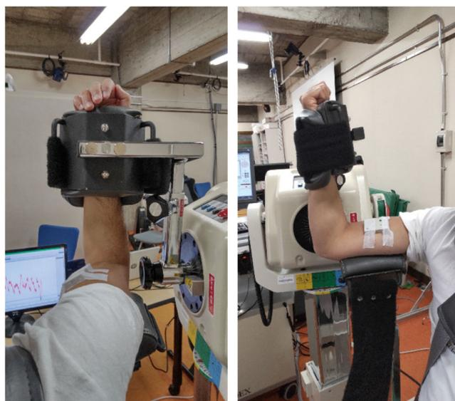
**FIGURE 2.** Overview of experimental setup. The subject was seated with arms slightly abducted from the trunk, elbow flexed at  $90^\circ$ , and forearm in a neutral position. The electrode was placed over the biceps brachii muscle.
